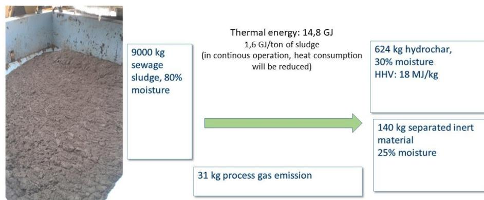
Figure 3. From Sewage sludge to biochar materials
