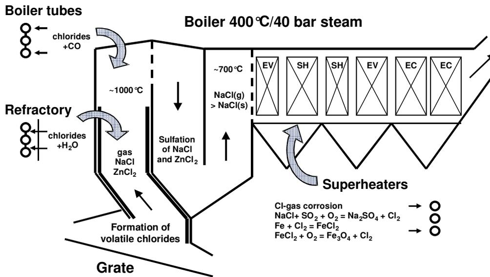
Figure 1. Typical corrosion problems in Waste-to-Energy plants
