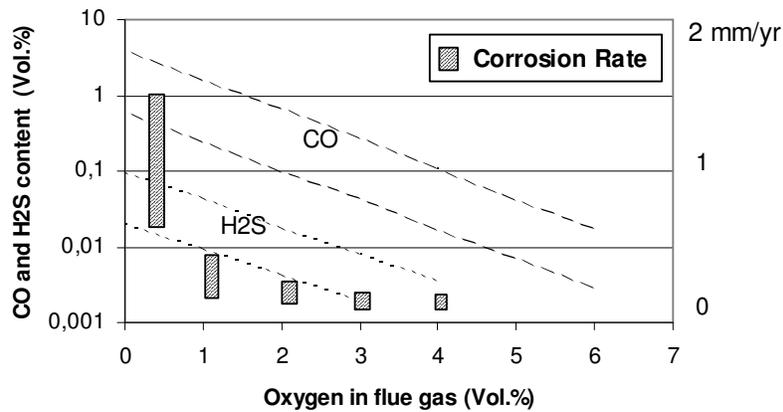
Figure 2. Corrosion of carbon-steel at 450° as a function of the flue gas composition in pulverized coal-fired boilers
