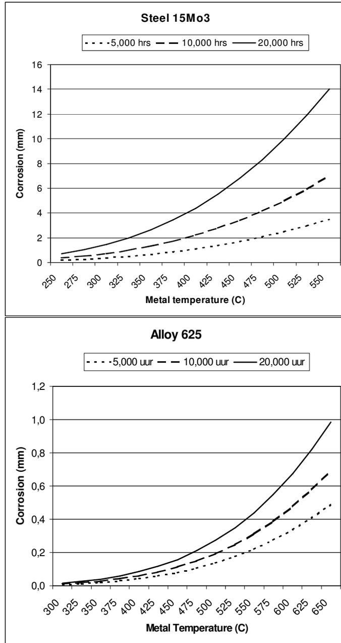
Figure 4. Extrapolated superheater corrosion data for boiler steel 15Mo3 and alloy 625 (18)
