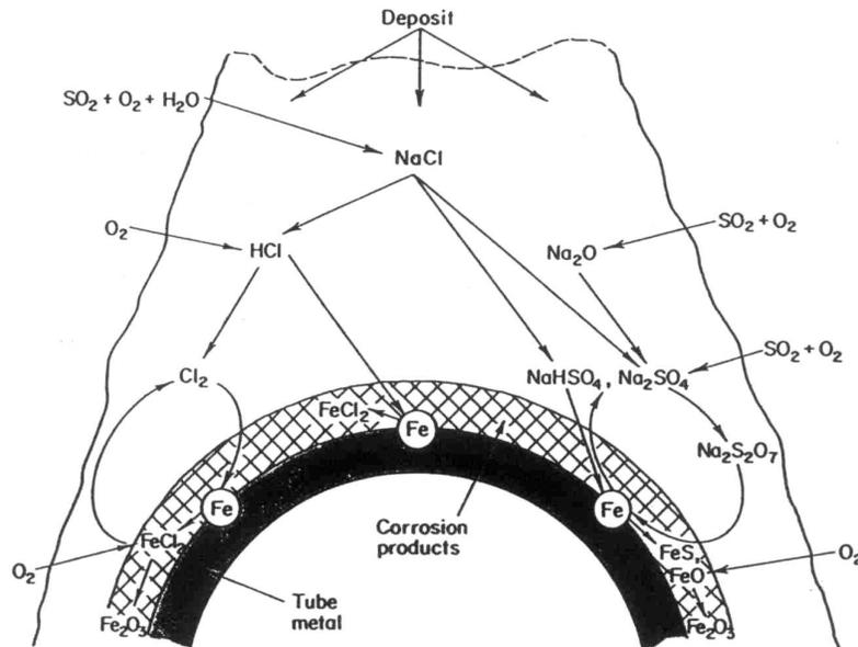
Figure 3. Sequence of chemical reactions explaining corrosion of incinerator boiler tubes (Ref. Krause, 1986, 1993)
