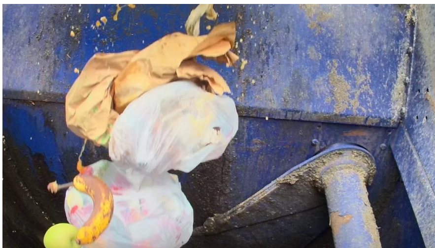
Figure 2. Food waste contaminated with plastics. The AI-based system detected the contaminants, captured an image, and recorded the data for analysis. Source: Östersund municipality.
