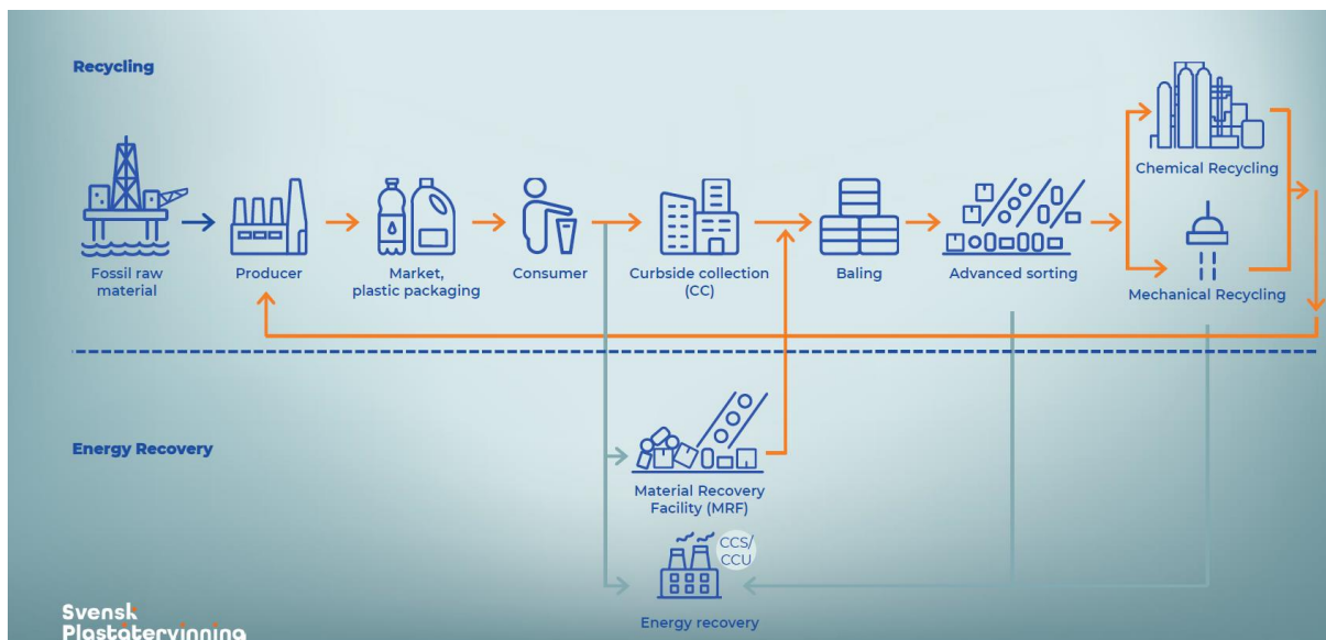
Figure 3. Site Zero recycling system scheme including the new units that might be added to the process in the coming years. Source: Svensk Plaståtervinning.
