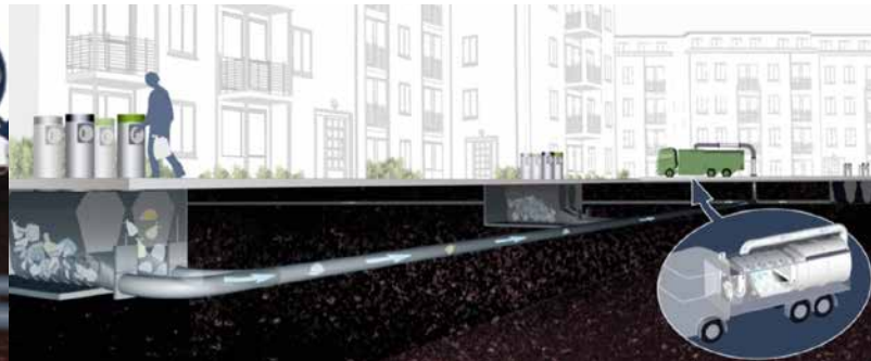
Figure 24: Picture of a mobile vacuum system (Source: Envac)
