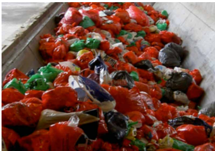
Figure 27: Optical sorting of multi colored plastic bags, Vänersborg AD plant, Sweden
