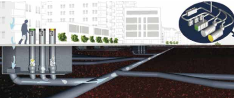
Figure 23: Picture of a stationary vacuum system (Source: Envac)
