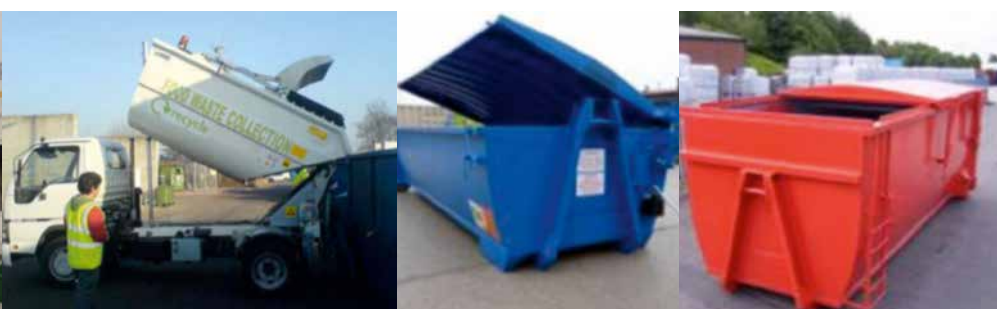
Figure 26: Bulking of organic waste in containers. Collection vehicle tipping (left) into a waste container (middle and right).
