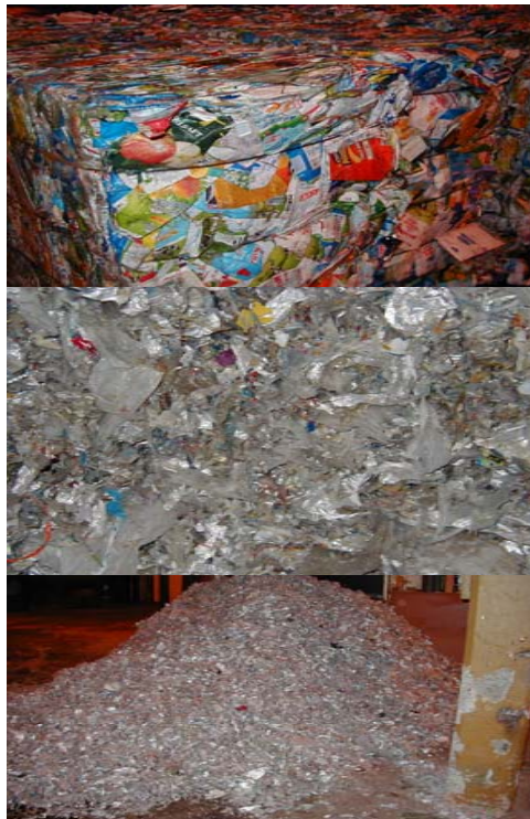
Plastic reject material with 10 % aluminium
