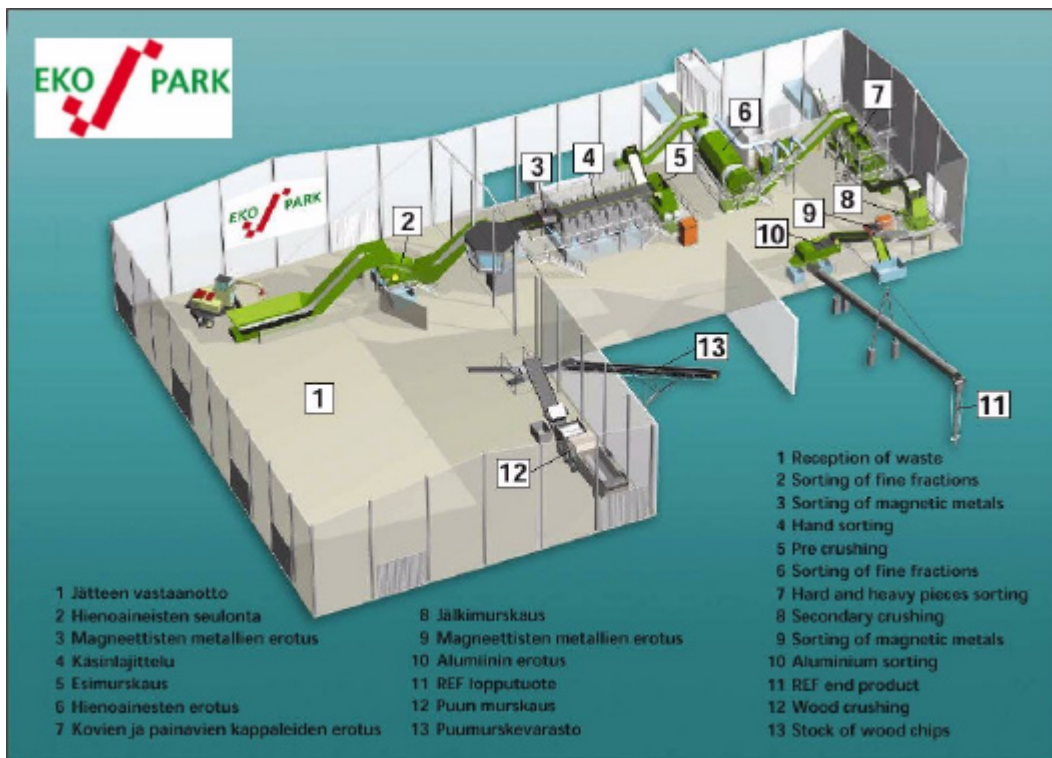
Figure 8. Processing of construction and demolition waste, Rakentajien Ekopark Oy.
