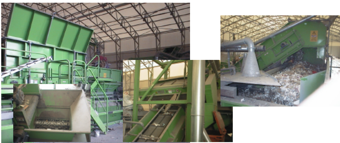
Figure 6. Processing of commercial waste: shredder, magnet and Eddy Current.
