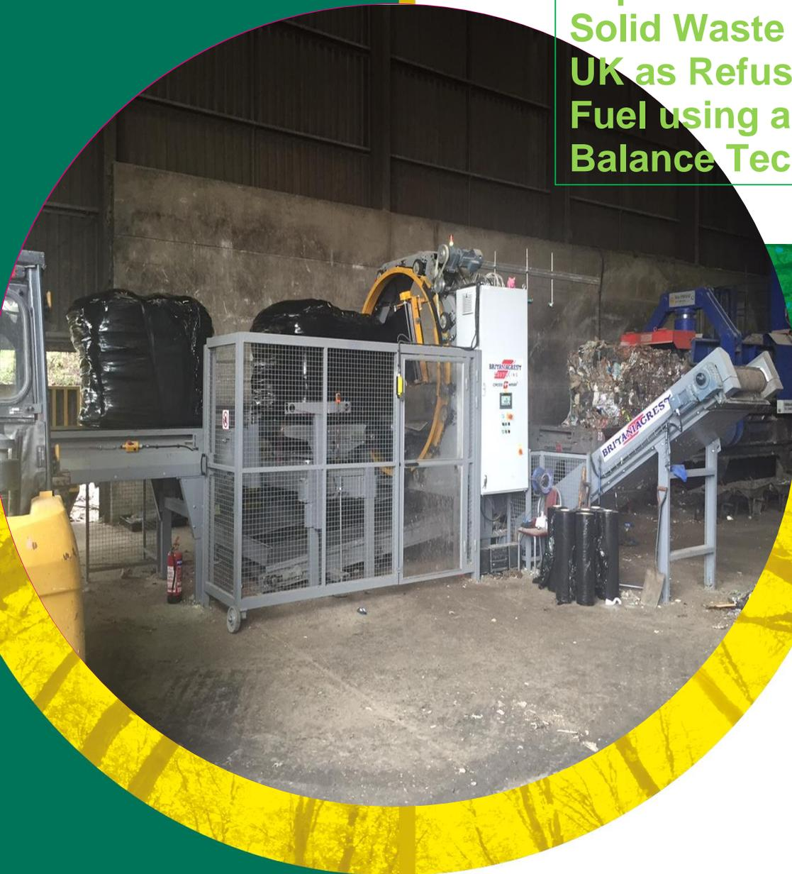
RDF being baled and wrapped in polythene protection prior to being loaded on transport for export from the UK.
