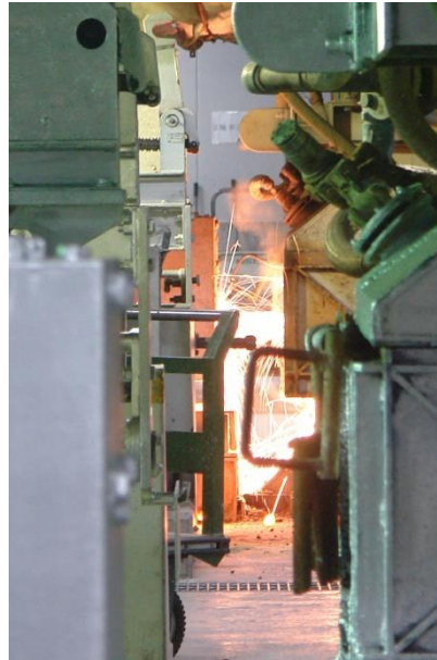
Figure A2.26: Discharge of liquid slag from furnace 2
