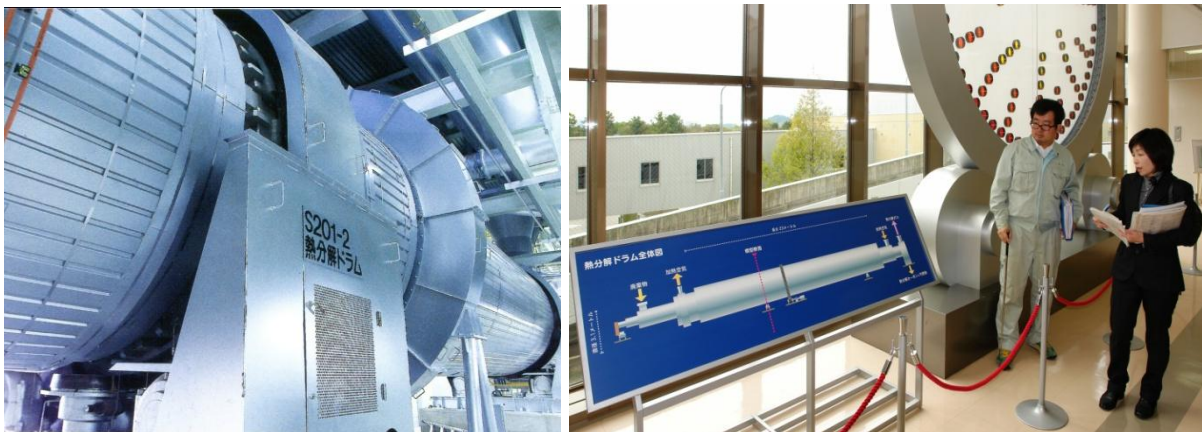
Figure A2.18: Photo of the pyrolysis drum (left) and of the operator explaining the function of the drum (right, with a full scale cross-section of the drum in the background)
