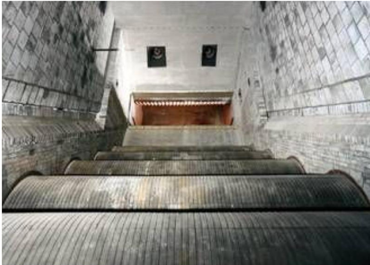
Figure 4.15: Combustion chamber with two lines of a horizontal grate (left) and five lines of a reverse-acting (right; adopted from [Martin 2009])
