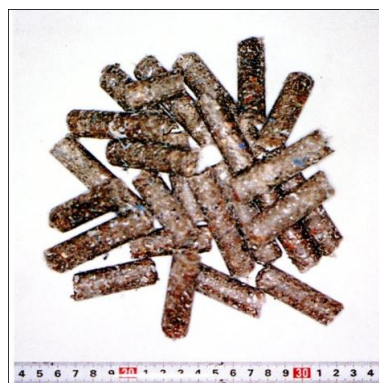
Figure A2.10: RDF pellets produced in the Omuta RDF processing plant
