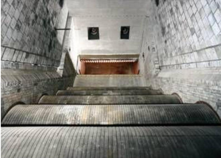
Figure 15: Combustion chamber with two lines of a horizontal grate (left) and five lines of a reverse-acting (right; adopted from [Martin 2009])
