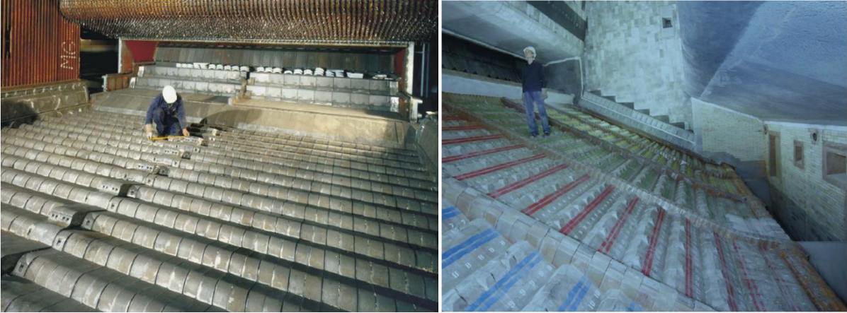
Figure 15: Combustion chamber with two lines of a horizontal grate (left) and five lines of a reverse-acting (right; adopted from [Martin 2009])
