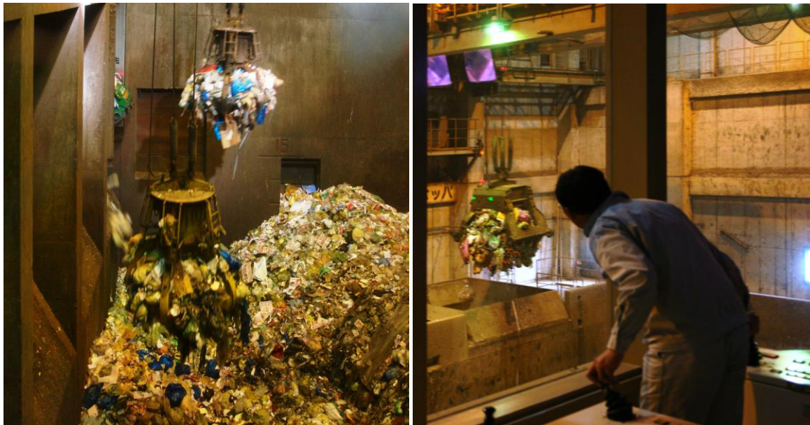
Figure 3: Waste bunker with two cranes mixing the waste (left) and filling the feeding hopper with a crane load of waste (right)
