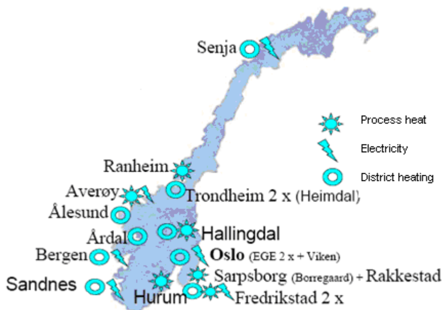
Figure 55: Plants generating energy from waste in Norway, 2009. Source: Rune Dirdal, Avfall Norge
